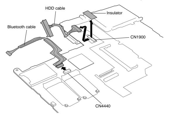
Figure 4-38 Removing the HDD cable/Bluetooth cable
